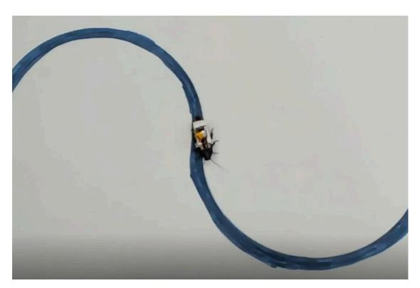
A new-generation electronic "backpack" can stimulate the cockroach by using 25 per cent less voltage than the previous iteration, while maintaining precise control of movement. PHOTO: NTU
